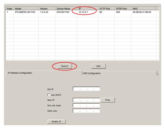
3. The IP Address for this device will display in the IP column.
