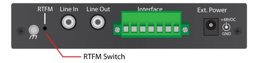
2. Continue to press the switch until after the indicator lights go off, and then release it. The VoIP Paging Gateway settings are restored to the factory defaults.
