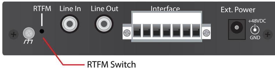
2. Continue to press the switch until after the indicator lights go off, and then release it. The Paging Adapter settings are now restored to the factory defaults.
