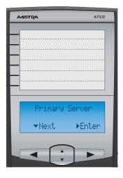
6. Enter the IP address of the PBX (Note: This IP can be either the Private or the Public IP address of the PBX, This depends on if the phone will be used locally or from a remote location.
