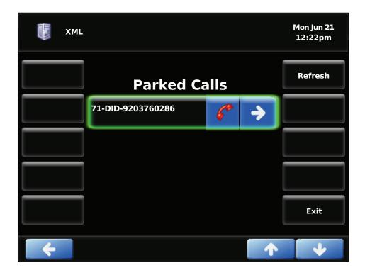
Using the up/down keys, you can highlight any caller and press the Pickup button to connect yourself with the caller.
