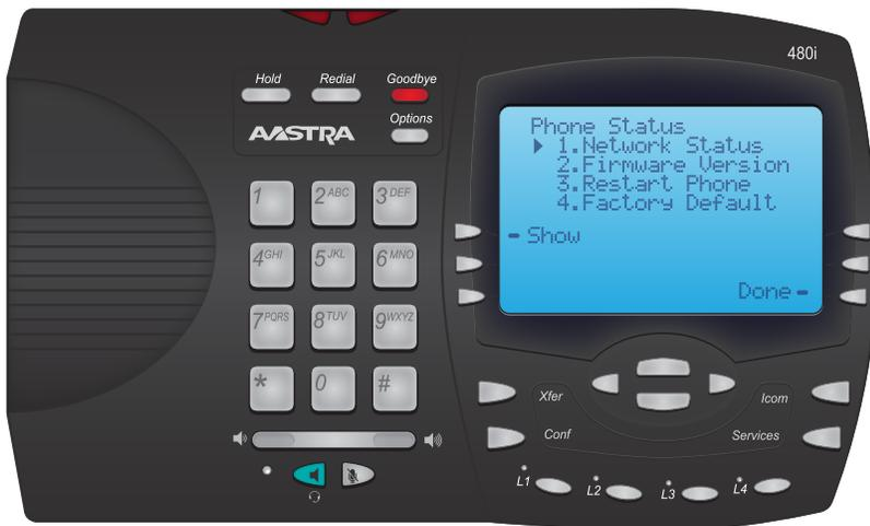
4. Using the left menu keys on the left hand side of the screen select the "IP ADDR" to see the IP address or "Mac Addr" to see the MAC address.
